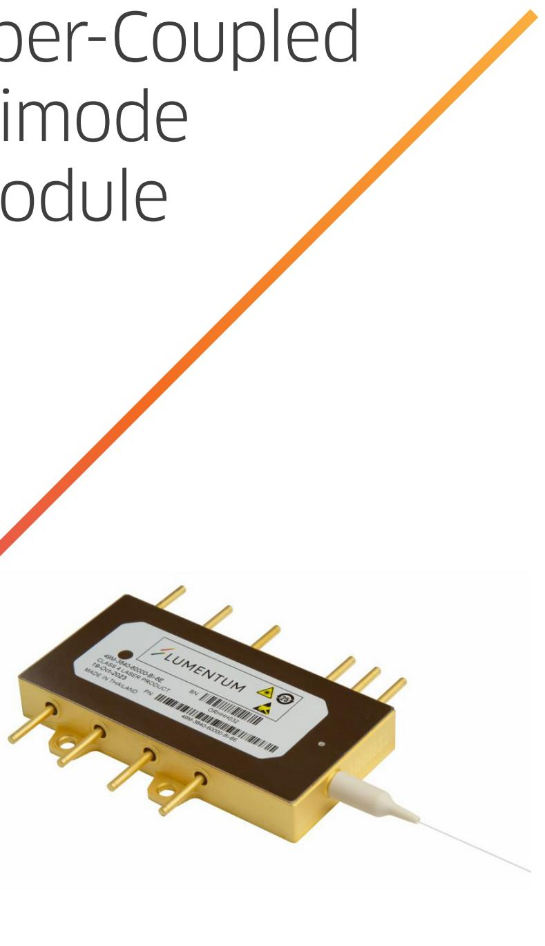
Lumentum's 49M Series diode lasers offer 40 W/60 W of power through a 105 $\mu$ m fiber. The 49M is a new platform that leverages the well-established and reliable designs of Lumentum's ST Series fiber-coupled diode lasers and the 4900 Series pump lasers.
