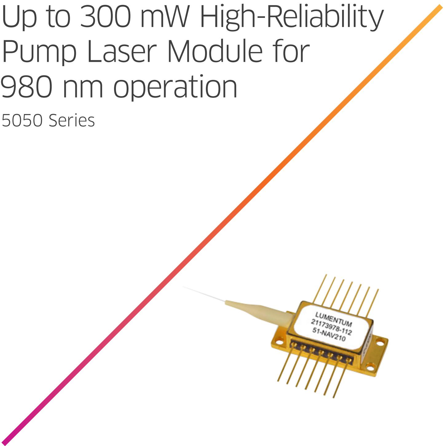
The Lumentum 5050 Series 980 nm pump laser module features low thermal impedance, a single-mode polarization-maintaining fiber output with a fiber Bragg grating (FBG) to stabilize the wavelength, and a hermetically-sealed 14-pin butterfly package.
