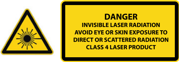
Laser radiation safety warning Laser classification per IEC 60825-1:2014 Maximum output power 2W
