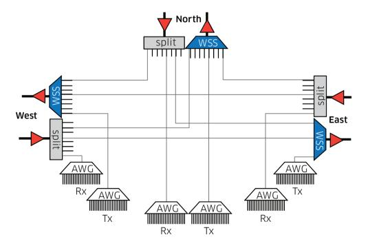
Figure 1. Broadcast-and-select node architecture with fixed add/drop
