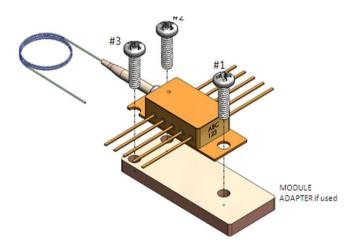
Figure 3. Bolting pattern for mounting a mini-BTF module
