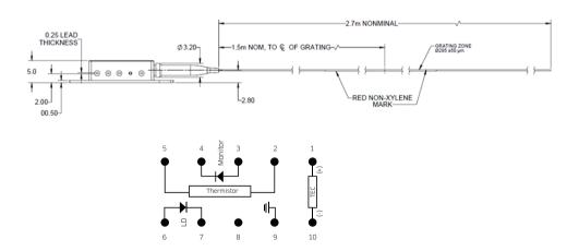
Figure 1 Top and side view and electrical schematic
