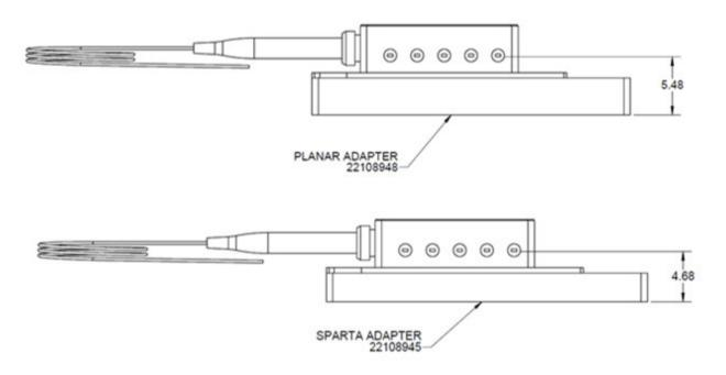
Figure 2. Side view of a mini-BTF module with spacer to match Planar or Sparta pin heights
