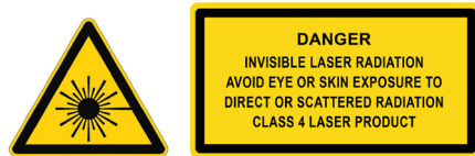
Laser radiation safety warning Laser classification per IEC 60825-1:2014 Maximum output power 2 W
